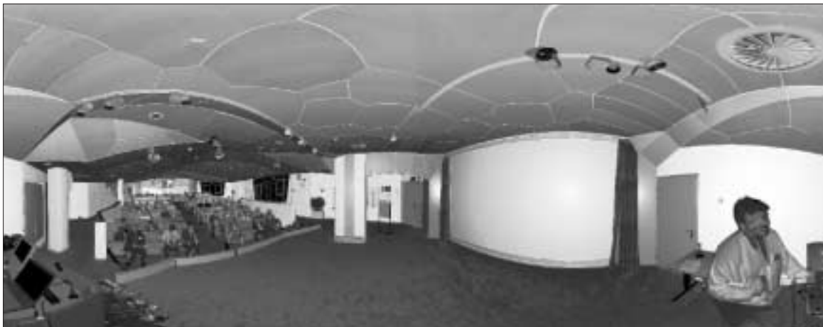
Figure 1: Scan acquired with a Z+F scanner of the lecture room with the intensity of the backscattered laser signal. The image shows the typical deformations of equal angle scans mapped onto a rectangular grid. In the foreground the podium can be seen with the presenter on the very right side. Left of the image center the audience is scanned (eye-safe).
