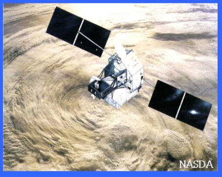
•TRMM and the world-first-space-borne Precipitation Radar (PR) enables to observe rainfall directly from the space.
