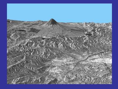
Mt. Fuji's terrain elevation map derived by JERS-1/SAR stereo.
