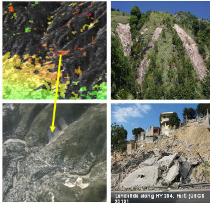
Figure 3 Monitoring earthquake triggered landslides affecting populated areas and transportation corridors in Haiti using RADARSAT 2 InSAR data (A).
