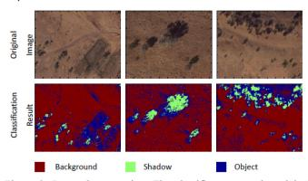
Figure 2: Image Segmentation: The classifier convert the original colour images into images with meaningful class labels.
