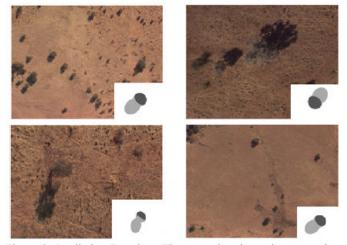
Figure 3: Predictive Template: The examples shown here are taken from different times during the flight. On the appearance model the darker area correspond to the object whereas the lighter area corresponds to the shadow. It can be seen that the relative position of the object and shadow is predicted correctly, also the ellipsoid shape assumption of the target is valid. Note that the templates are not plotted to the true scale.
