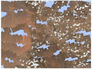
Figure 6: Detection results over a selected mission area, the white circles are the points of detection, multiple circles occasionally shows up for the same tree because the same tree crown was detected in separated frames. The individual image frames are joint together using algorithm described in (Bryson, 2010)
