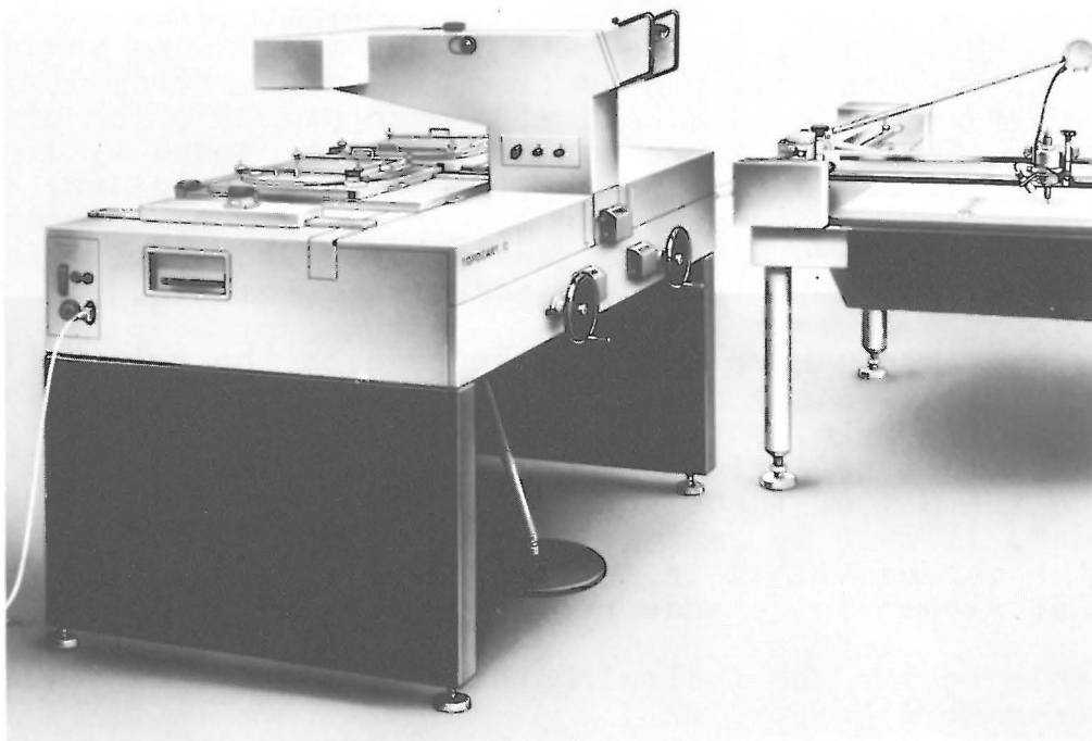
Fig. 1: TOPOCART C Stereoplotter
