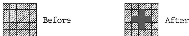
Figure 1 Ground Model Modification Scheme for Marking Control Points (Each square represents a brightness value stored in the ground description).
