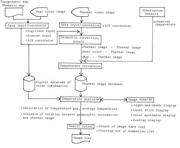
Fig. 7 Flow of processing
