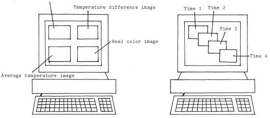
Fig. 4 Screen display function used for temperature analysis
