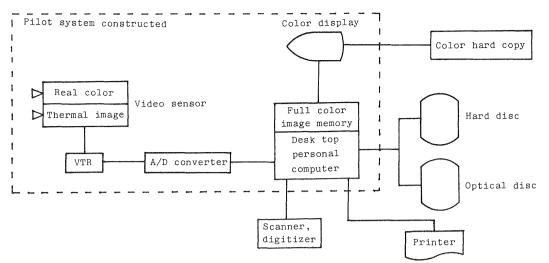
Fig. 5 Hardware configuration
