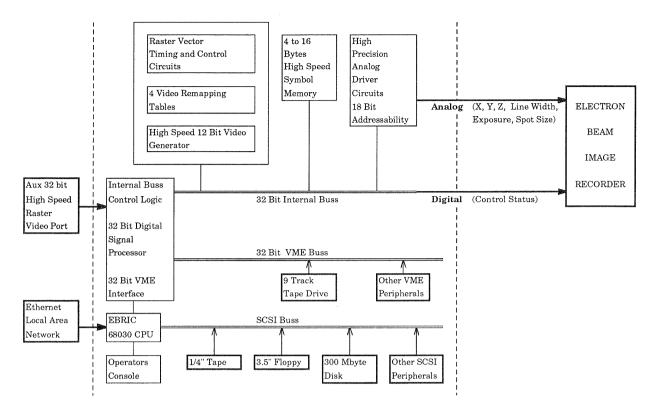
Figure 2 Block Diagram of RVG 450
