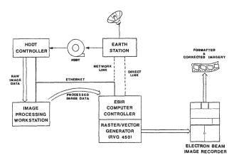
Figure 1 EBIPS-3000 System Configuration
