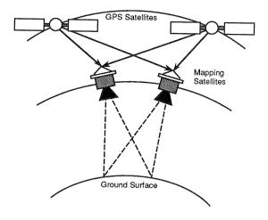
Figure 7: Concept of spatial stereo-mapping from space in real-time.
