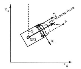
Figure 4: Transformation of relative positions determined with the stereo-vision system into the absolute coordinate frame.
