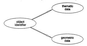
Fig. 3. Information structure for representation of terrain objects.
