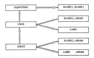
Fig. 5 Class and superclass structure of objects.
