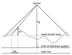
Fig. 2: Displacements  $\Delta s$  caused by terrain height differences  $\Delta h$
