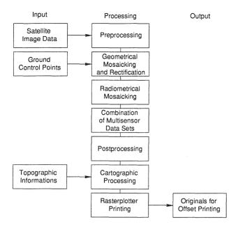
Fig. 1: The production line for Satellite Image Maps
