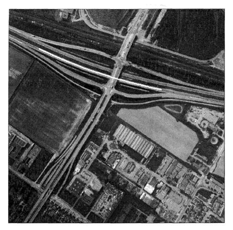
**Fig. 2** Blue band of a scanned colour aerial photograph, pixelsize 1.60 m., representing the present situation. The considered road segment from the database is superimposed on the image in white.
