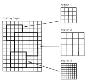
FIG. **3.** Regions comprising a single layer are dynamically resampled to a uniform raster definition when displayed.
