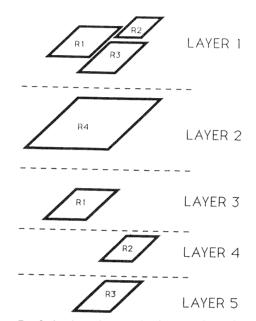
Fig. 2. A schematic example of a raster image in CARIS composed of four regions (R1-R4) and five layers.
