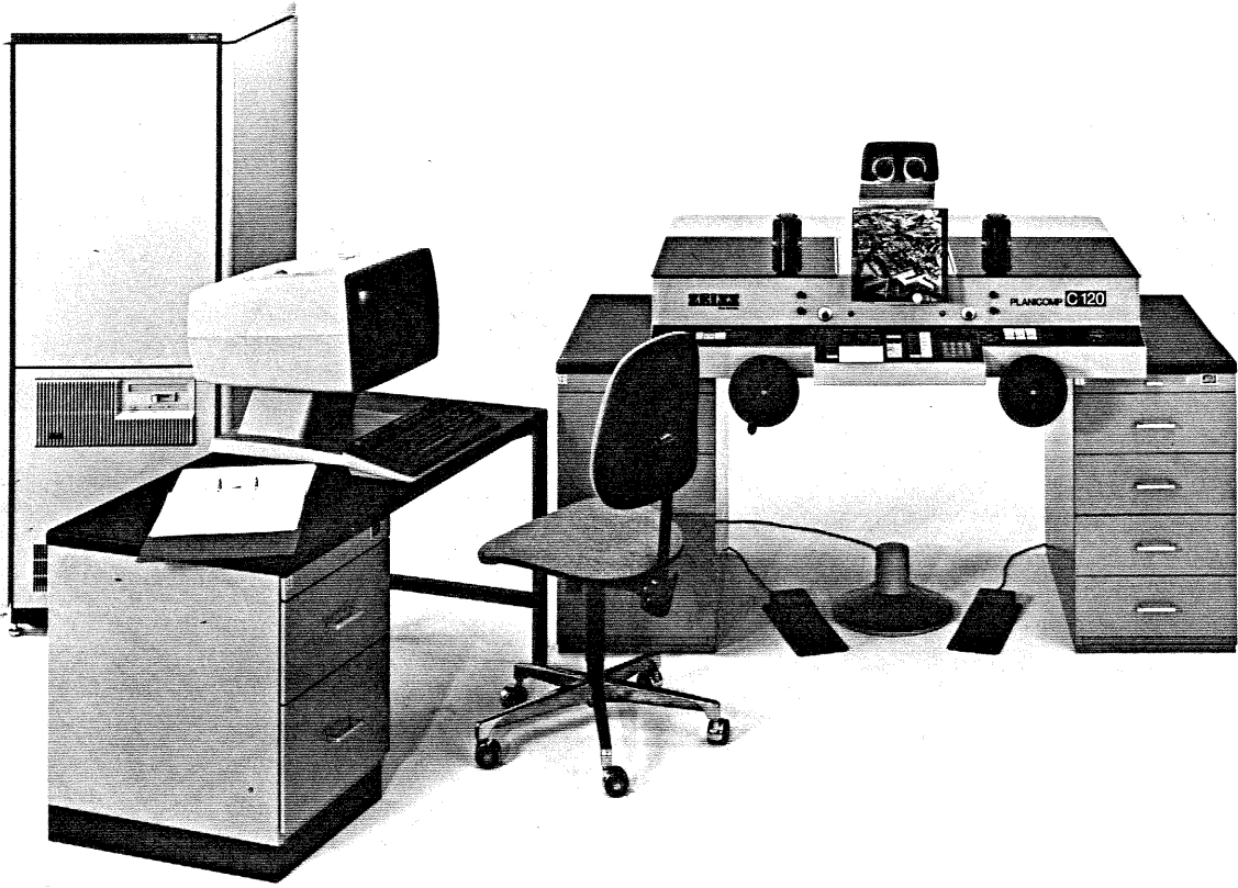
Fig. 1: C120 Planicomp with Zoom Viewer and HP 1000 A700 Computer
