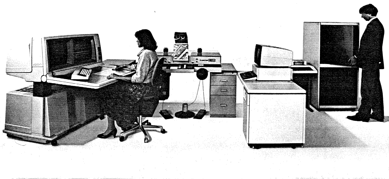
Fig. 4: Interactive Mapping with the Zeiss Planicomp and the Intergraph Stereodigitizer Workstation
