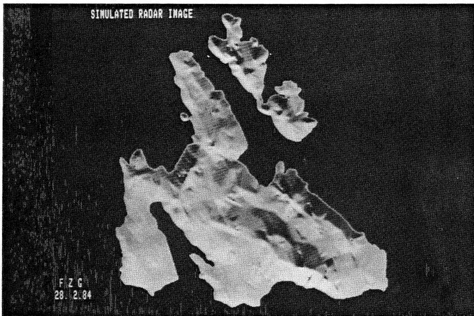
Fig. 4 : Simulated radar image using imaging and sensor parameters from SIR-A recordings and stereo-derived digital elevation model.
