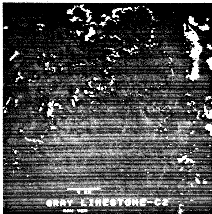
Fig. 9 - Illustration of Supervised Classification (Maximum likelihood algorithm) of the C 2 unit (Bambuí Group) which hosts fluorite mineralizations.
