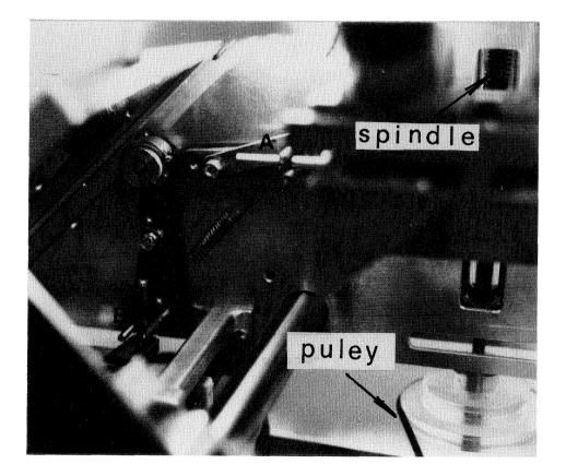
Figure 5 - The mechanical triangle AOB has been realized, avoiding any possible backlash and reducing the frictions to a minimum extent.
