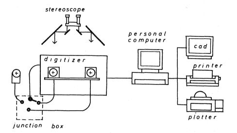
Figure 1 - The modified Rolleimetric System
