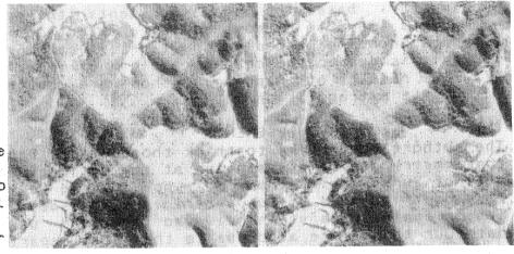
realization of Figure 5 air photo stereo pair fully automatic measurement of parallaxes.Two ways of automatic method of locating corresponding point pairs are possible: one is the methods used in automatic registeration of remote sensed images[9];the other is recently developed namely "Feature based Corresponding Algorithm for Image Matching"[10]. The mapping method is also tested with aerial stereo images and
