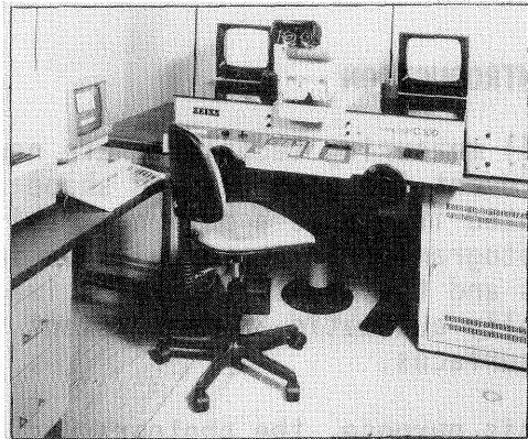
Fig. 2: InduSURF plotting system, comprising C100 Planicom, HP 1000 host computer, A 900 and CCD module
