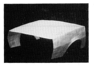
Fig. 5. Measured car model part B-spline surface of degree 3.
