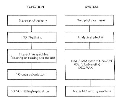
Fig. 1. Overview of the production system and the apparatus and software used.
