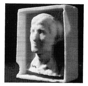
Fig. 4. N.C. milled surfaces of a face. Left: scale 1:1, B-spline surface of degree 3, hard foam. Right: scale 1:2, B-spline surface of degree 3, soft foam.
