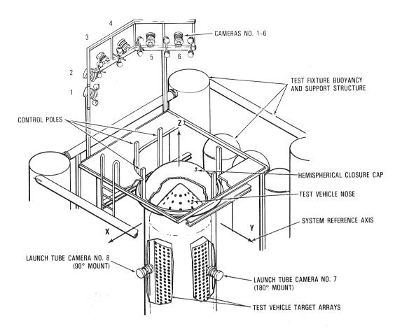
Figure 1: Test fixture assembly
