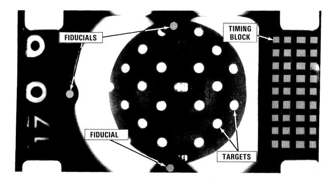
Figure 5: Photograph of TV resection targets as seen by camera #7
