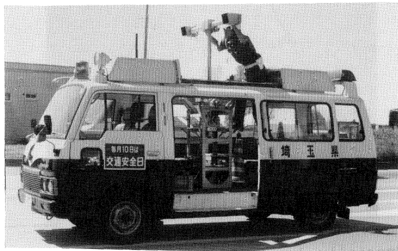
Mechanism for raising/lowering a stereocamera ( Courtesy of Saitama Prefecture Police Hqr. )
