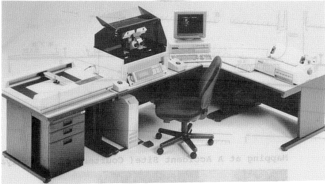
PAMS ( Photogrammetric Analytical Measurement System )
