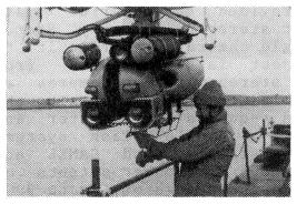
FIGURE 4. A pair of CI7070 cameras mounted on a small ROV.
