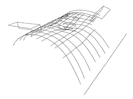
FIGURE 6. Perspective drawing of dented pipe with outline of corrosion pipes. Scale bars are also shown.
