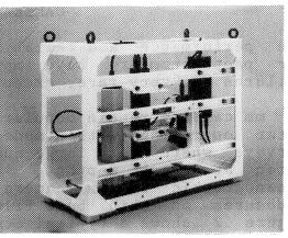
FIGURE 2. Typical CAMEL oceanographic photographic system.
