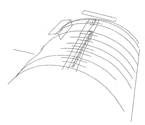
FIGURE 7. Perspective drawing of damaged pipe.
