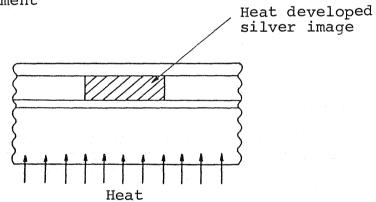
Figure 1 Exposure and development in dry-printing
