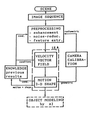
Fig.1 : Basic process in motion analysis
