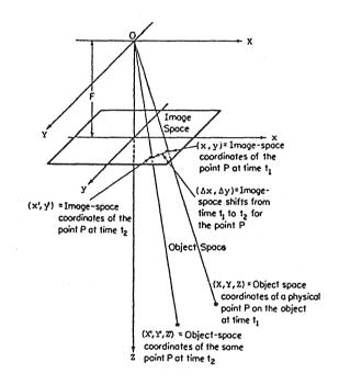
Fig.2: Basic geometry in 3-D motion estimation
