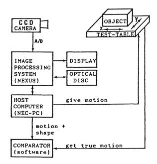
Fig.3: Experimental system for verifiable experiments in motion analysis
