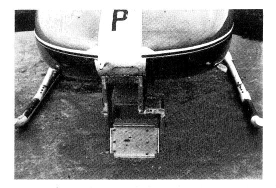
Figure 5. The Nose Mount for the Hasselblad Camera on the Helicopter
