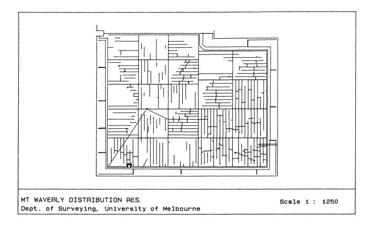
Figure 3. Surface Cracking and Jointing in the Mt Waverley Distribution Basin
