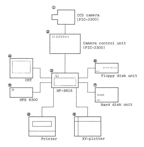
2. Automatic crack analysis system
