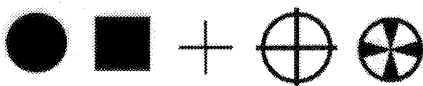
Figure 1: A collection of possible measuring marks digitized on a DTP scanner. From left to right: circular mark; quadratic mark; cross-hair; circled cross-hair; cross-hair with arrows.
