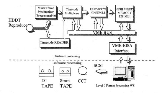
Fig.4: Block diagram of the programmable formatter system
