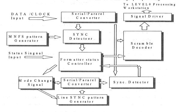
Fig.1: Block diagram of MOS-1 MESSR hardware synchronizer.
