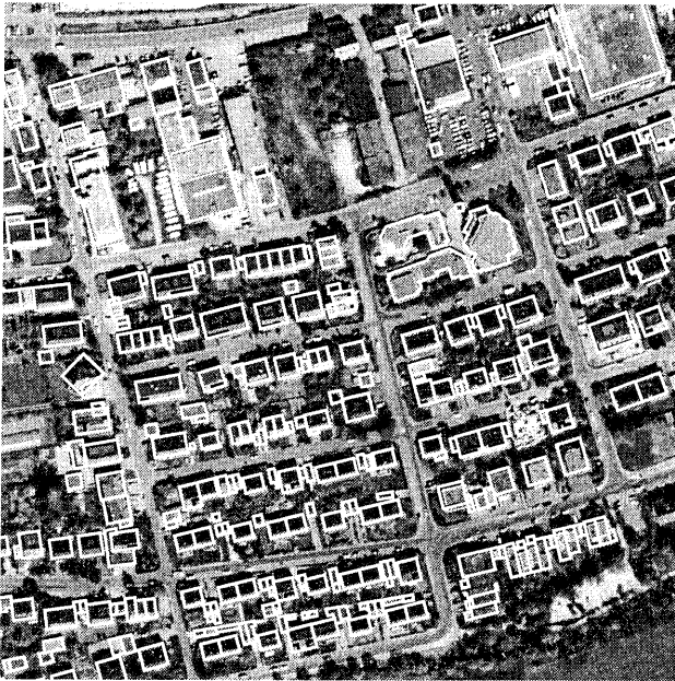
Figure 4: Image section with projected ground plans.
