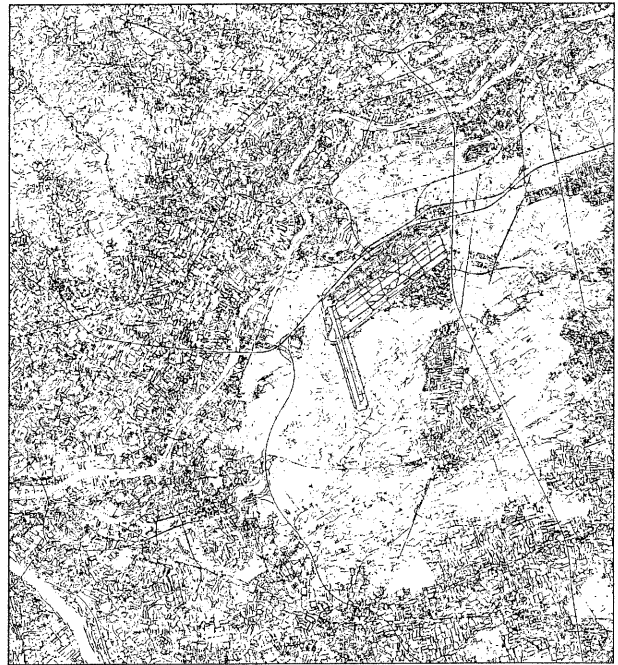
Figure 6: Lines extracted from the SPOT XS data (Fig. 4) using a window size of 5 \times 5 pixels.
