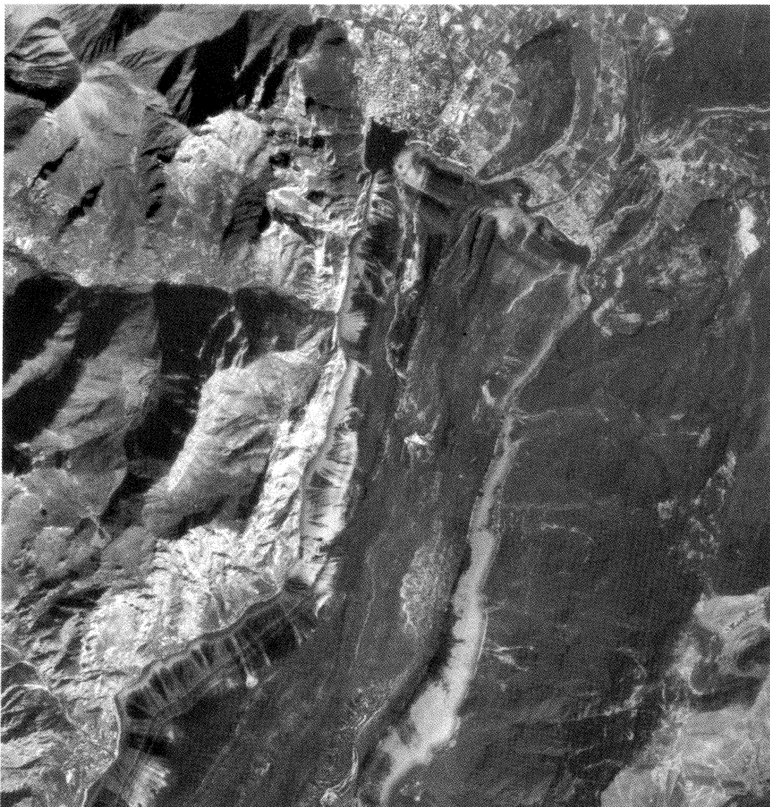
Figure 7 - Two-dimensional view of the upper part of Lake Garda basin. In this illustration the sidescan sonar image of the lake's bottom has been merged with an onshore digital orthophoto to obtain a continuous view of the terrain as if the water of the lake were removed from the image.
