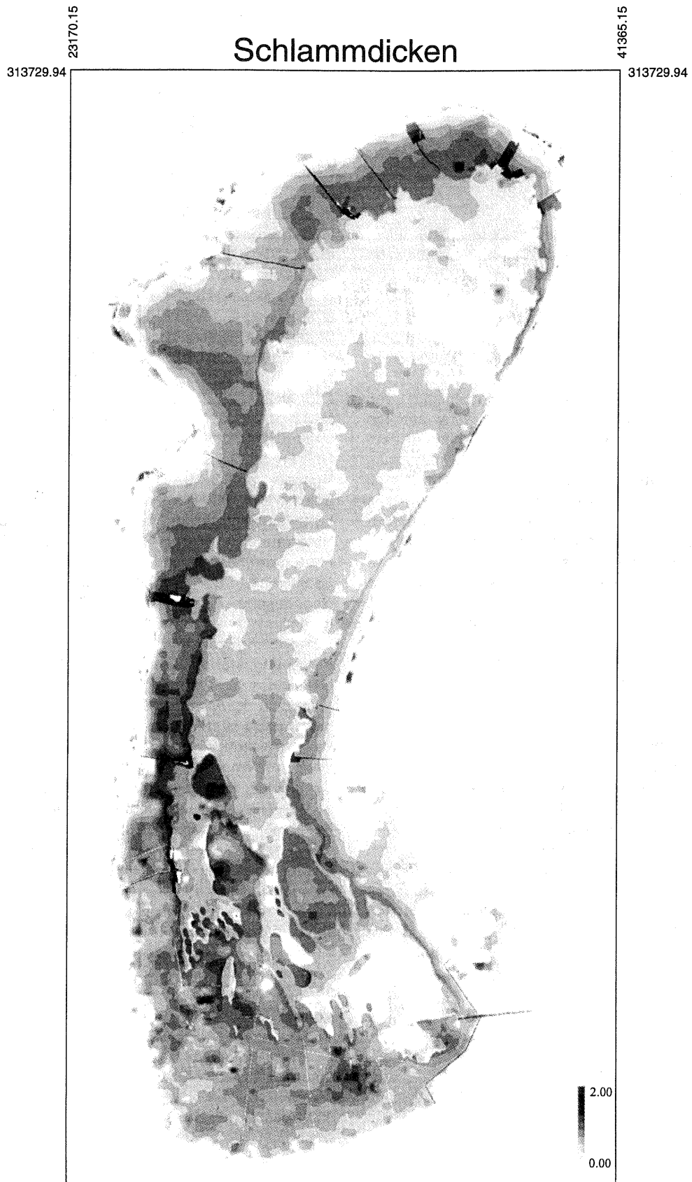
Figure 1. Digital model of sediment thickness of the bottom of Lake Fertő, scale \approx 1:180000 .
