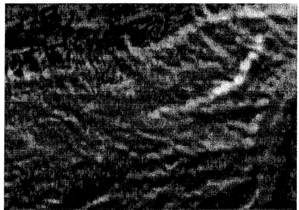
Figure 6. Day-time TM band 6 image adjusted for effects of solar heating
