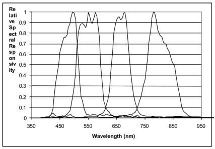
Figure 4 Normalized multispectral filter response
