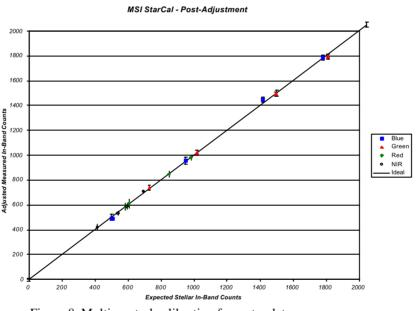
Figure 8 Multispectral calibration from star data
