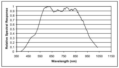
Figure 2 Pan CCD relative spectral response
