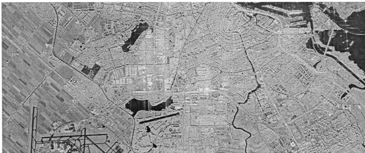
Figure 1. Example of a fully polarimetric PHARUS image of Amsterdam and Schiphol. The colors are assigned in the following way: HH channel to red, HV+VH to green and VV to blue.
