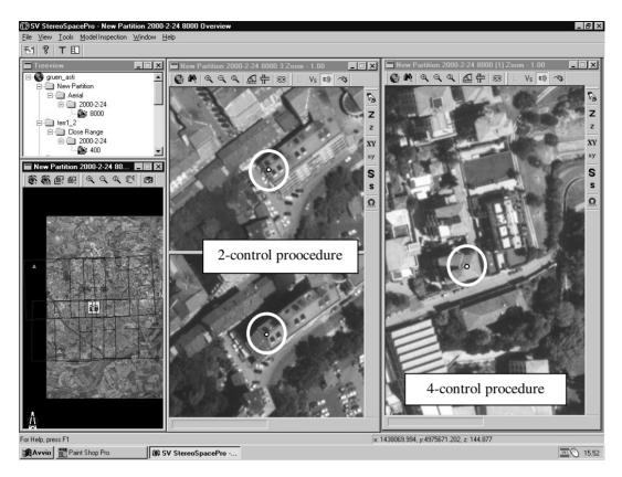
Figure 8. Stereoscopic collimation of single points in an aerial block
