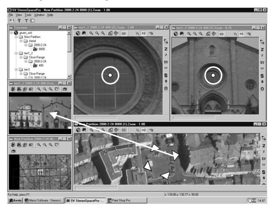
Figure 7. Hot-spots joining aerial and terrestrial blocks
