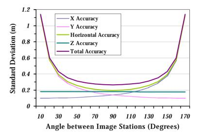
Figure 5: Simulated Ground Point Standard Deviation – 2 Images, Sensor Configuration D, 10 m from feature
