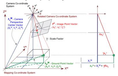
Figure 2: 3-D Co-ordinate Calculation using Georeferenced Images
