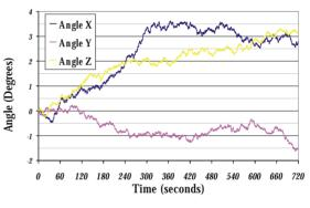
Figure 1: Angular Drift from Low-cost Strapdown IMU (Crossbow DMU-FOG)
