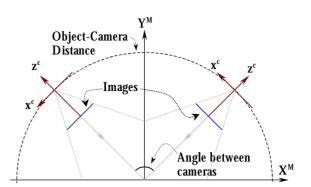
Figure 4: Imaging Geometry for Simulations
