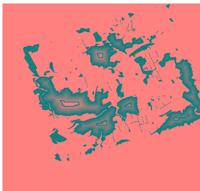
Figure 8. Distance image from projected GIS objects and seed regions from reduced GIS objects
