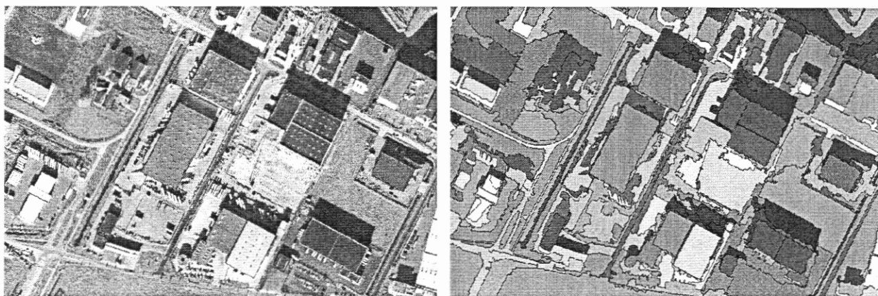
Figure 3: Result of segmentation: original nadir data set (left, resolution: 50 cm), and segmented image (right).
