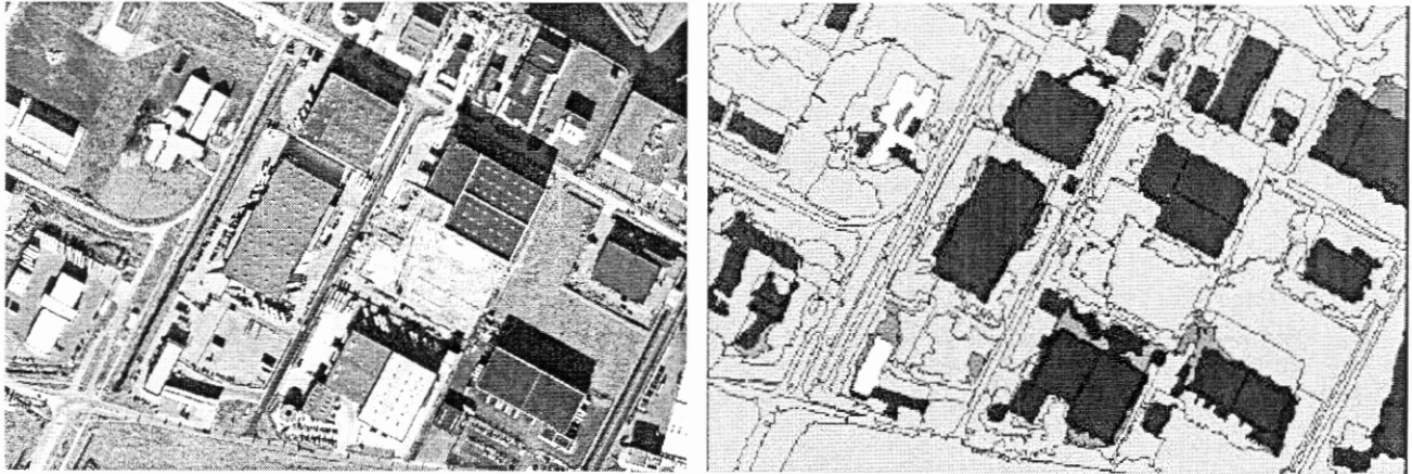
Figure 4: Nadir image with rasterised vector data set (white) (left) and house detection (white: houses in the vector data set, light grey: low areas, dark: new houses, dark grey: low classification probability (shadows))
