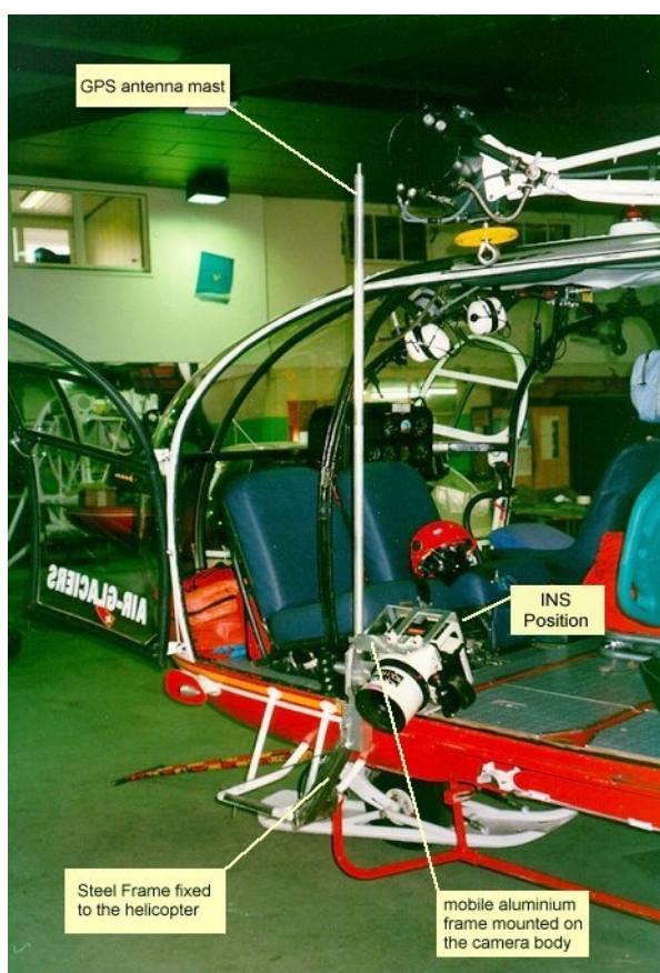
Fig.4: Global view of the system mounted on the helicopter Alouette III.
