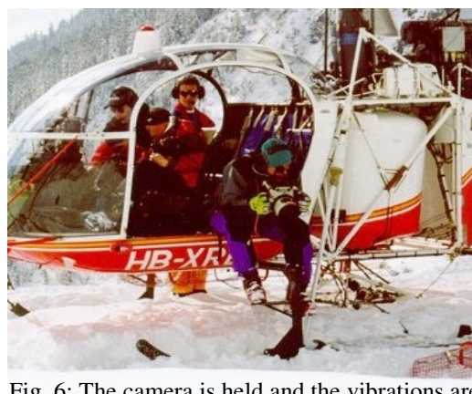
Fig. 6: The camera is held and the vibrations are dampened by the body of the operator.
