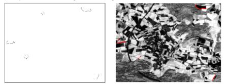
Figure 6: Matched points of map-image pixels (left) and SPOT subscene registered to the map (right).
