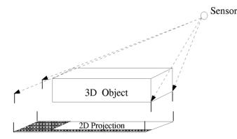
Figure 3: A model of perspective distortion.
