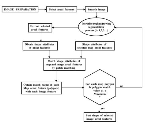
Figure 2: Algorithm for extracting selected image features with best shape.
