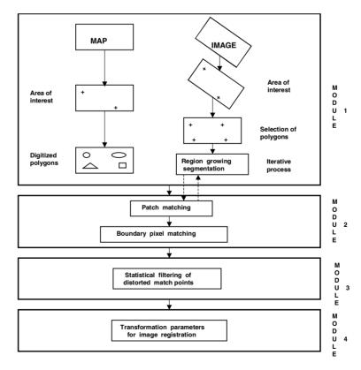
Figure 1: The ARMIES system for automatic map-image registration.
