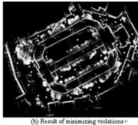
Figure 6: Result of multiple registration when location and direction of range images are unknown.
