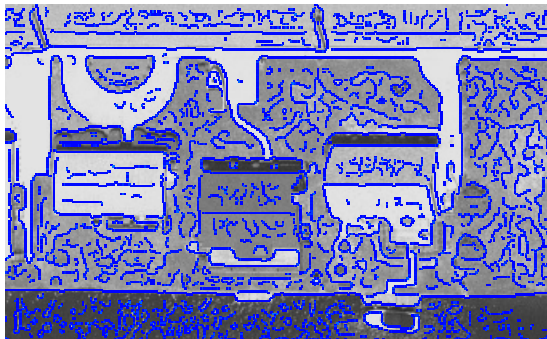
Figure 3. Aerial image and detected edge pixels.
