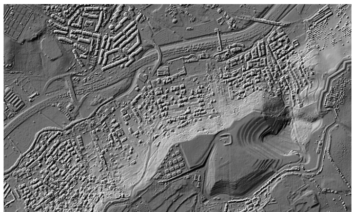
Figure 6. Portion of a Shaded DEM of Lisbon (Portugal), processed by ISTAR (France) using HRSC-A Data
