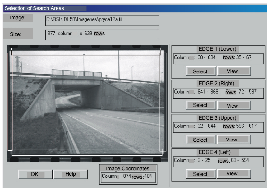
Figure 3. Selections of search areas for format edges. Main window of the non-metric images inner orientation program under I.D.L. 5.0.
