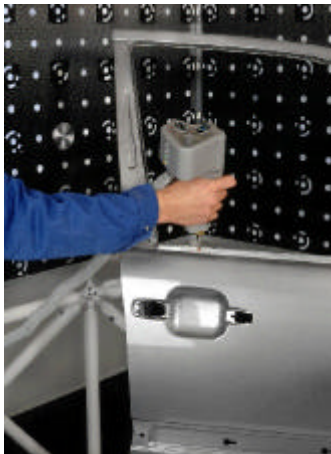
Figure 5: On-line measuring system with active probe orientation (AICON Procam 3 )
