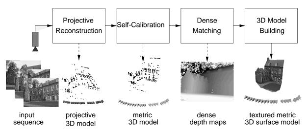
Figure 1: Overview of the system (the cameras are represented by little pyramids, the results of the dense matching are accumulated in dense depth maps where light means close and dark means far).
