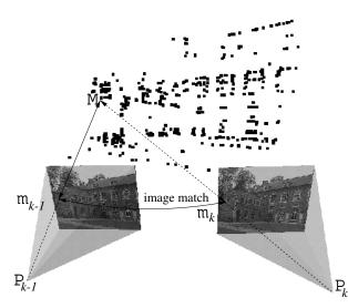
Figure 2: Image matches  $(m_{k-1}, m_k)$  are found as described before. Since the image points,  $m_{k-1}$ , relate to object points,  $M_k$ , the pose for view k can be computed from the inferred matches  $(M, m_k)$ .
