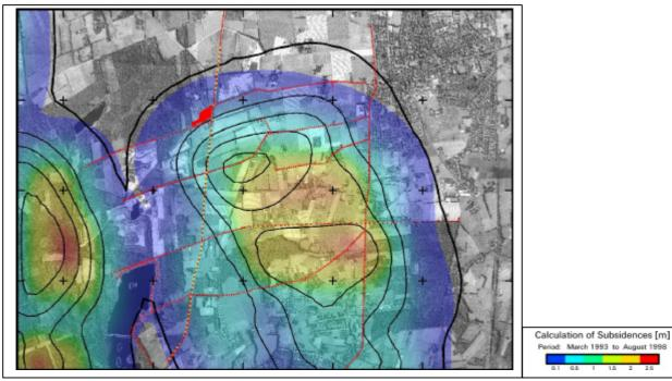
Fig. 2: HRSC-A orthoimage August 1998; "Calculation of Subsidence 1993-1998"; red: GPS-points 1999; yellow: levelling points; black: 1 m-contour-lines "Calculation of Expected Subsidence 1993-2004"
