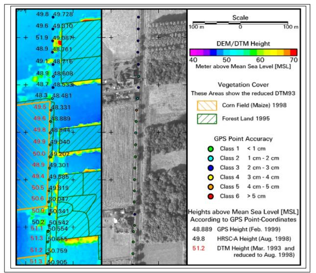
the GPS heights (see Fig. 7). In this specific case it is clear that for planar and non-vegetated areas the HRSC-A DEM is more accurate than the subsidence calculations.
