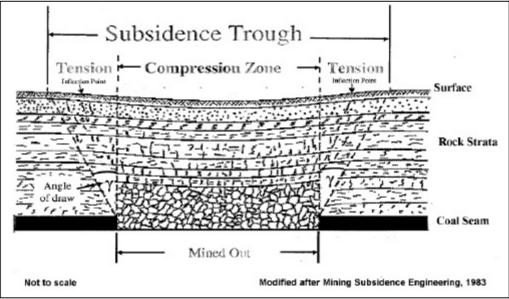
Fig. 1: Cross-section of subsidence trough
