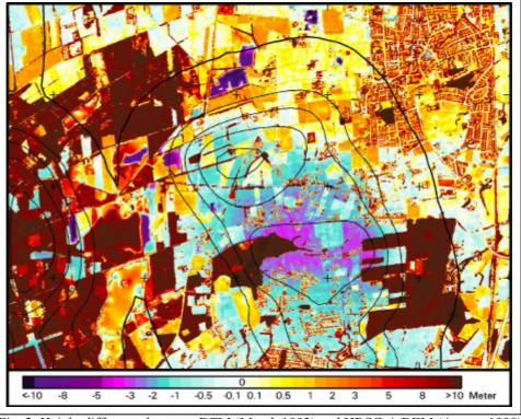
Fig. 3: Height difference between DTM (March 1993) and HRSC-A DEM (August 1998)
