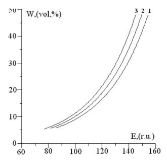
Fig.1 Water content in vol% as a function of the scatterometer intensity E calculated using a priori data on the soil texture of the Chernobyl area. (1) is sandy (2) sandy loam and (3) is loamy soil.
